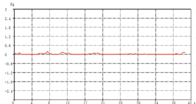
Fig. (10). Resistance at the speed of 0.1m/s in transverse test mode.
