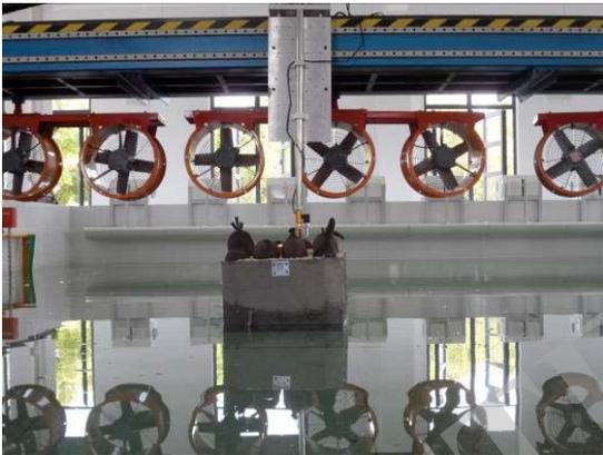
Fig. (2). Transverse towing test by constant speed.
