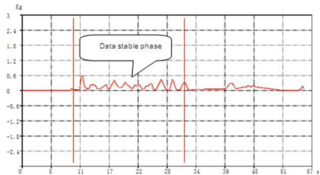
Fig. (12). Resistance at the speed of 0.3m/s in transverse test mode.
