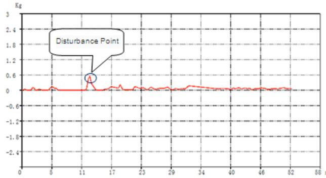
Fig. (11). Resistance at the speed of 0.2m/s in transverse test mode.
