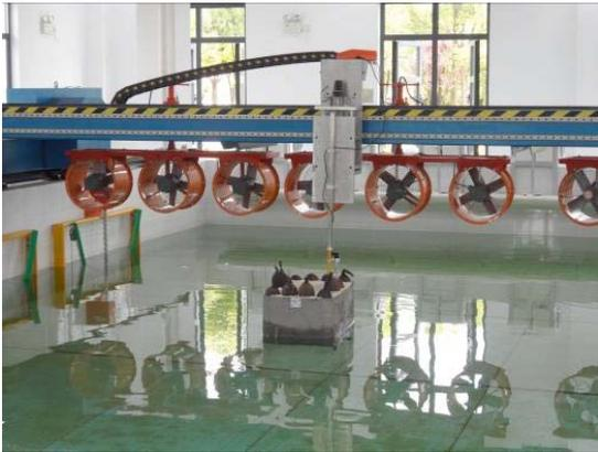
Fig. (1). Straight towing test by constant speed.
