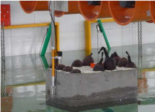
Fig. (5). Force cell fixed on trailer.
