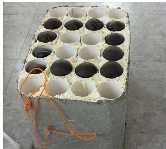
Fig. (4). The open caisson physical model.
