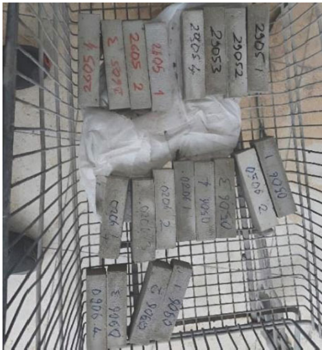
Fig. (4). Specimens prepared for compressive and flexural strength testing.
