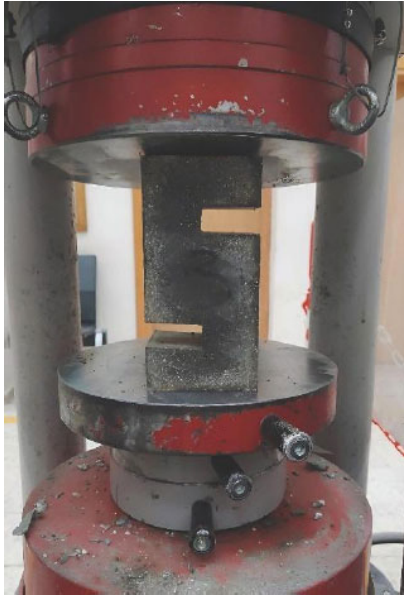
Fig. (6). Shear strength testing apparatus and setup.
