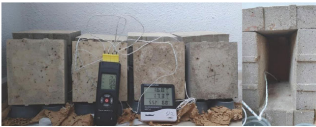
Fig. (7). Thermal performance monitoring setup.
