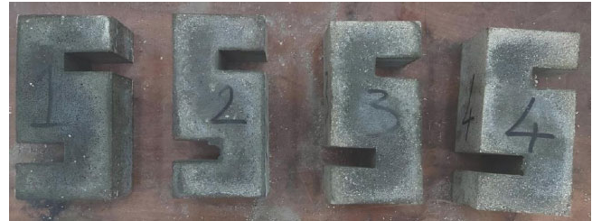
Fig. (5). Specimens prepared for shear strength testing.
