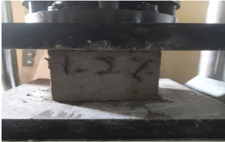
Fig. (3). A concrete cube in a compressive test machine.
