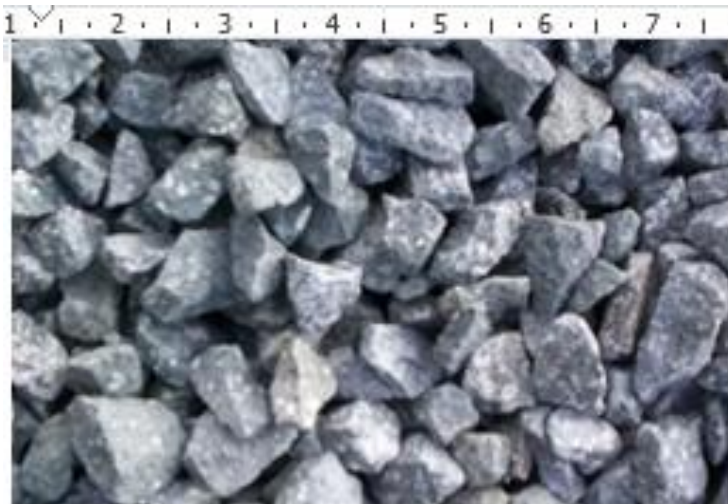
Fig. (1). Granite for concrete coarse aggregate.
