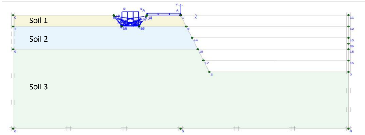
Fig. (6). Factor of Safety of the critical slope in the basic condition.
