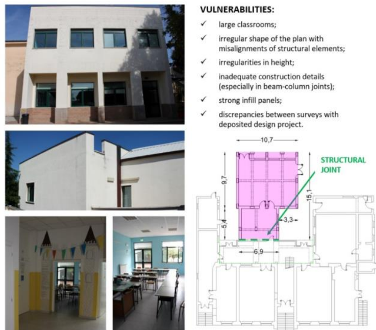
Fig. (3). Photographic views and the list of vulnerabilities of the analysed school building.
