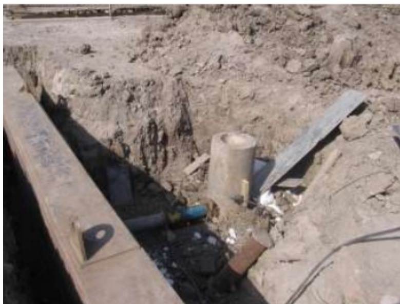
Fig. (2). Field test diagram of horizontal loading test.
