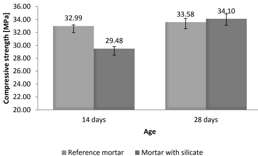
Fig. (7). Compressive strength of reference mortar and mortar with 30% vol. LAR, for calculation of Pozzolanic Activity Index.
