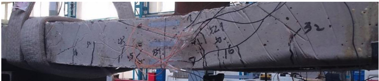
Fig. (19). JM-1 CFRP debonding breakage.
