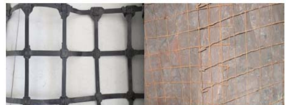
Fig. (1). The physical map of steel plastic geogrid and metal net.
