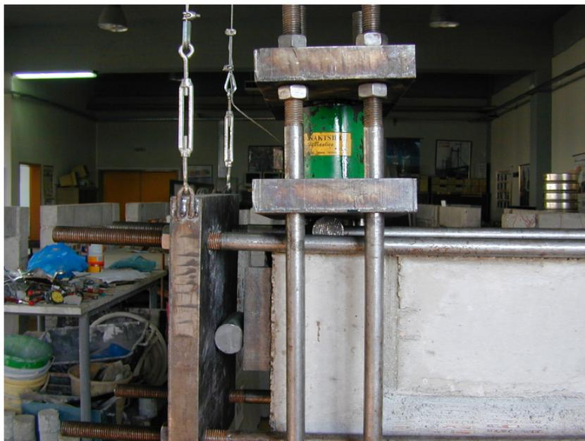
Fig. (4). Roller implementation for the application of the vertical and horizontal frame forces.
