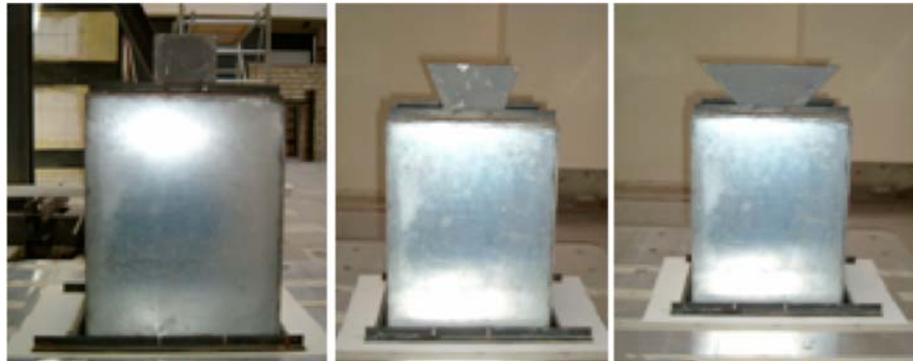
**Fig. (3).** Rigid structural prototypes with tanks of different shapes and liquid depths.
