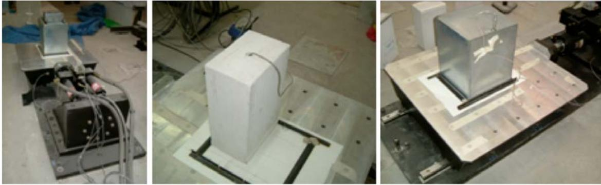
**Fig. (2).** The shaking table and the rigid blocks used during experiments.
