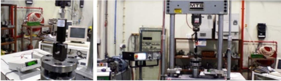
**Fig. (4).** Magneto-rheological damper with current supply device connected to MTS universal setup.
