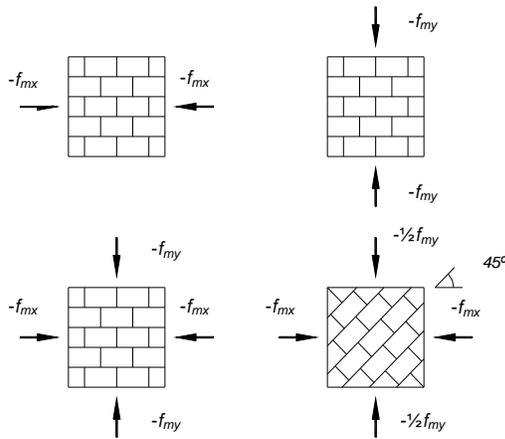
**Fig. (3).** Separate tests required to calibrate an anisotropic model. (a) uniaxial compression parallel to the bed joints (b) uniaxial compression perpendicular to the bed joints (c) coupling parameter between normal stress values in the case of compressive failure (d) coupling parameter which weights the shear stress contribution to compressive failure.
