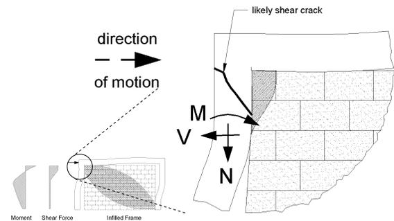
**Fig. (10).** Action effects induced in the reinforced concrete column due to the interaction with the masonry infill panels.
