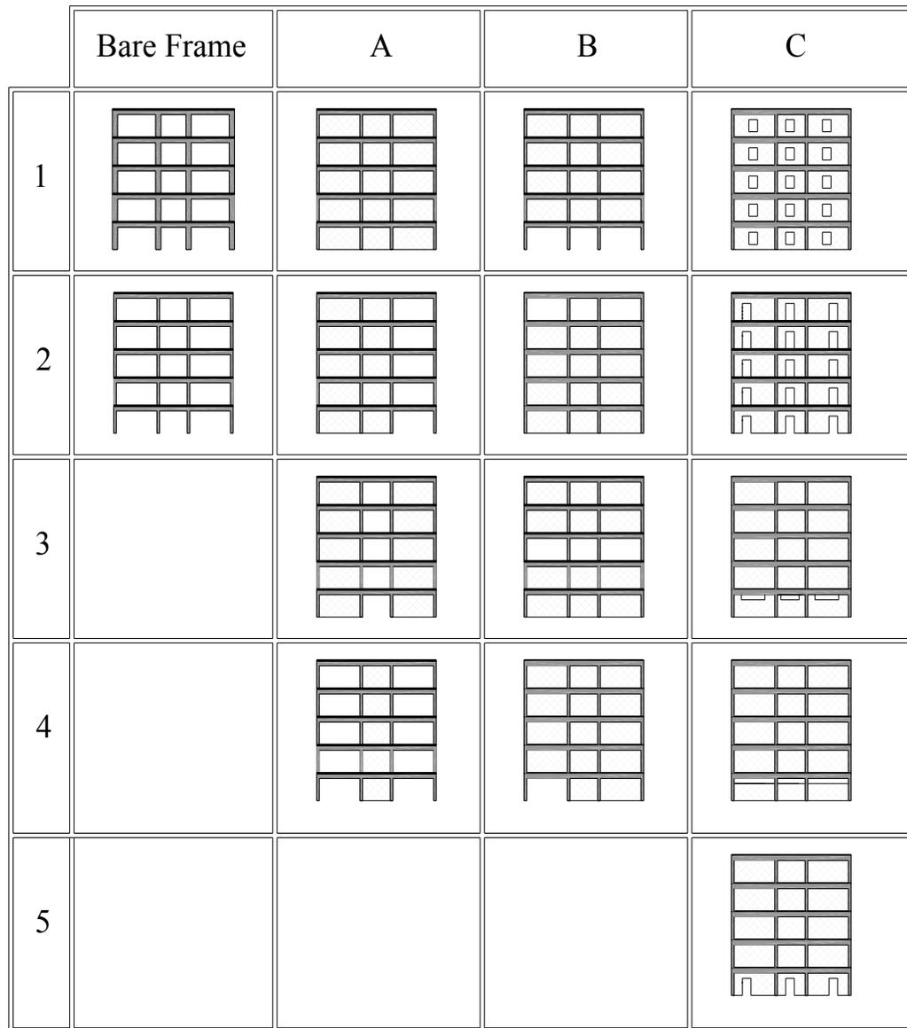
Fig. (18). Different structural configurations for infill distribution layout.
