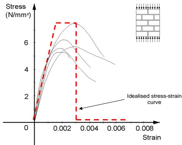
**Fig. (2).** Schematic idealisation of a typical stress-strain curve for brickwork masonry in compression, overlaid on particular stress strain curves for different masonry types, as reported in [8].
