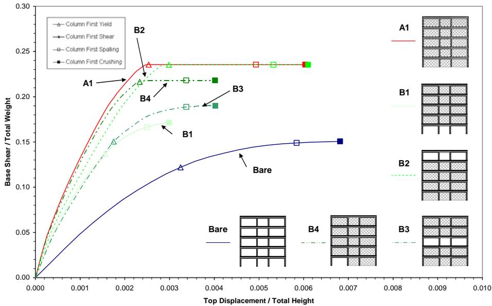
Fig. (24). Capacity curves – B series weak frame.
