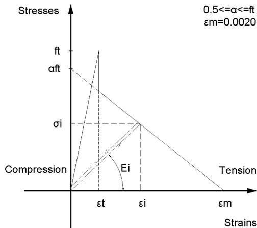
Fig. (6). Tensile strain softening model implemented together with loading and unloading.
