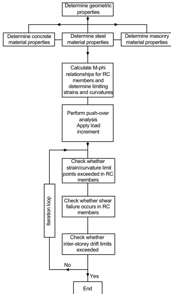
Fig. (9). Schematic flow-chart of the assessment methodology.
