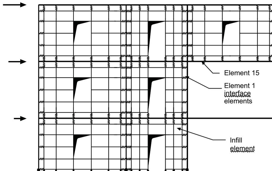
**Fig. (8).** Graphical representation of a typical numerical model of a LE-MIRCF construction using the aforementioned elements.
