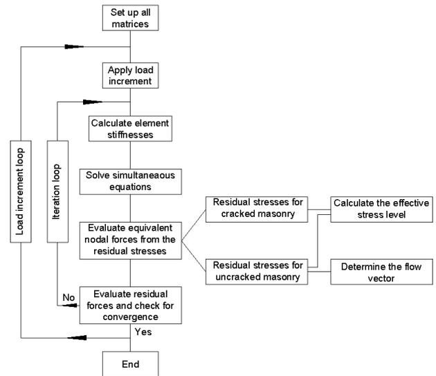
**Fig. (7).** Flow chart highlighting the steps implemented within the overall program solution procedure in order to account for the inclusion of the masonry infill element.
