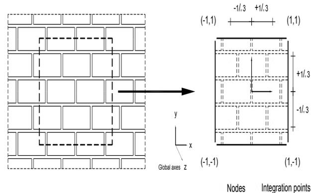
**Fig. (1).** The representation of the masonry infill panel is achieved by considering a single finite element to represent several bricks and mortar joints. The typical 4-node membrane element is also shown with the locations of the nodes and integration points, corresponding to a 2 x 2 rule (all coordinates are shown normalised).
