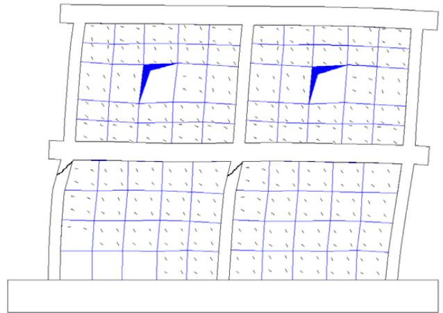
**Fig. (14).** The final deflected shape as obtained from the simulation also showing membrane cracking and RC shear failure.
