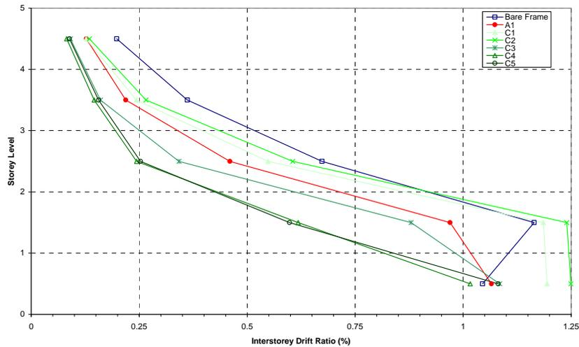
**Fig. (28).** Inter-storey drifts at the ultimate displacement for the C series weak frame.
