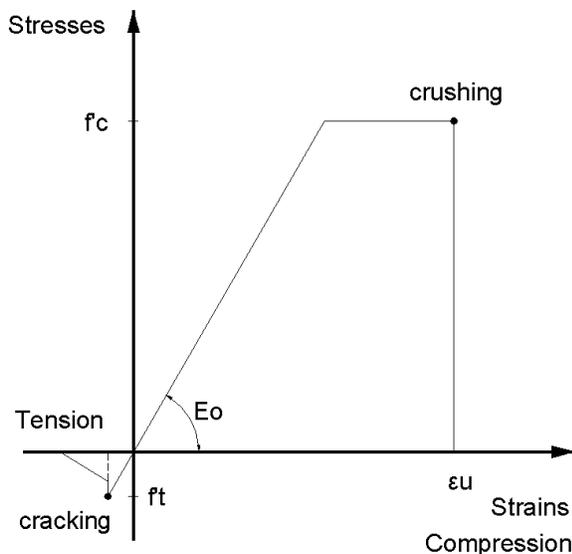
Fig. (5). The masonry constitutive model.
