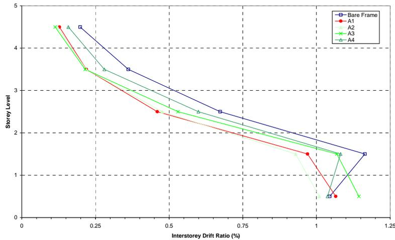
Fig. (22). Inter-storey drifts at the ultimate displacement for the A series weak frame.
