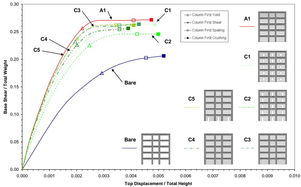
Fig. (26). Capacity curves – C series strong frame.
