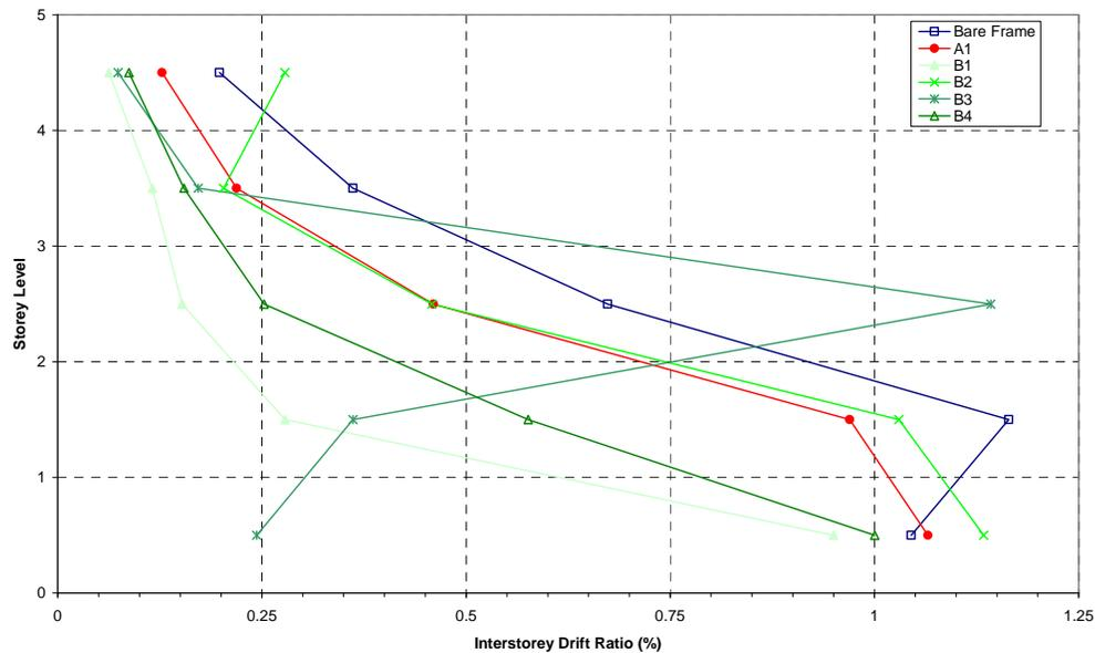
**Fig. (25).** Inter-storey drifts at the ultimate displacement for the B series weak frame.
