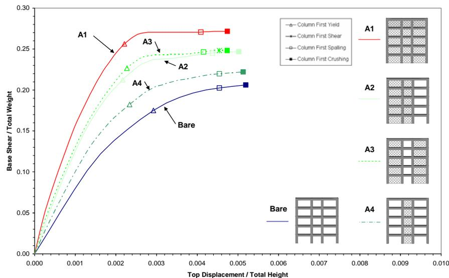
**Fig. (20).** Capacity curves – A series strong frame.
