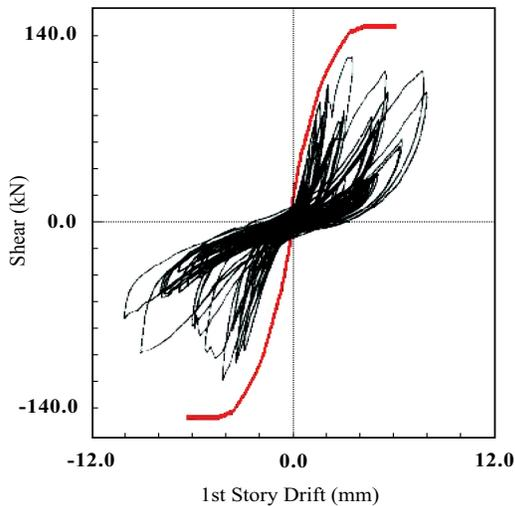
**Fig. (13).** The overall structural response in terms of the load versus displacement diagram for the experiment by Buonopane and White [40], and that of the simulation.
