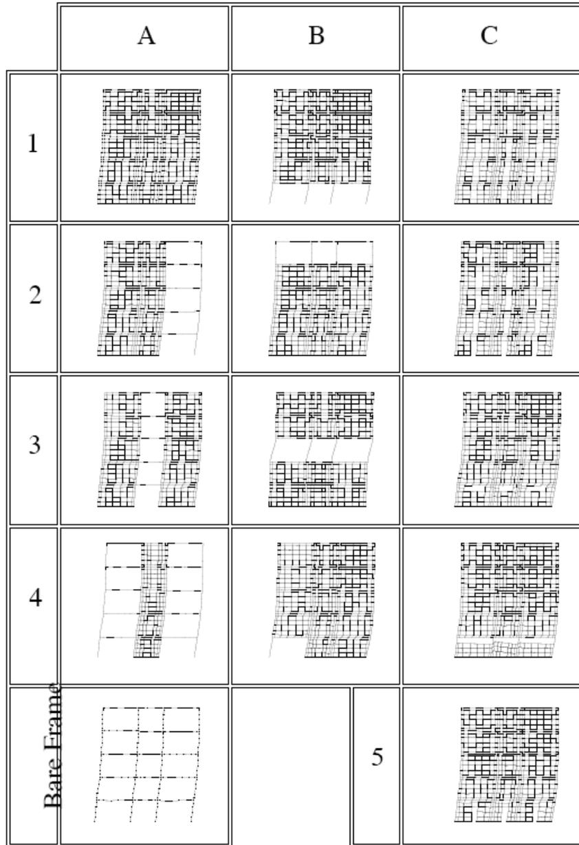
**Fig. (19).** Final displaced shapes for the weak frame assemblages.
