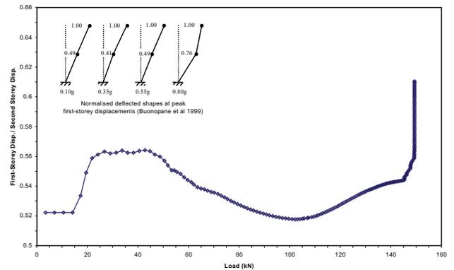
**Fig. (17).** Ratio of inter-storey drifts predicted during the simulation clearly showing the development of a soft storey mechanism and agreeing with the recorded experimental results shown in the inset [40].
