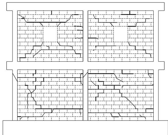
**Fig. (15).** The final crack pattern following the 0.80g test as reported by Buonopane and White [40].
