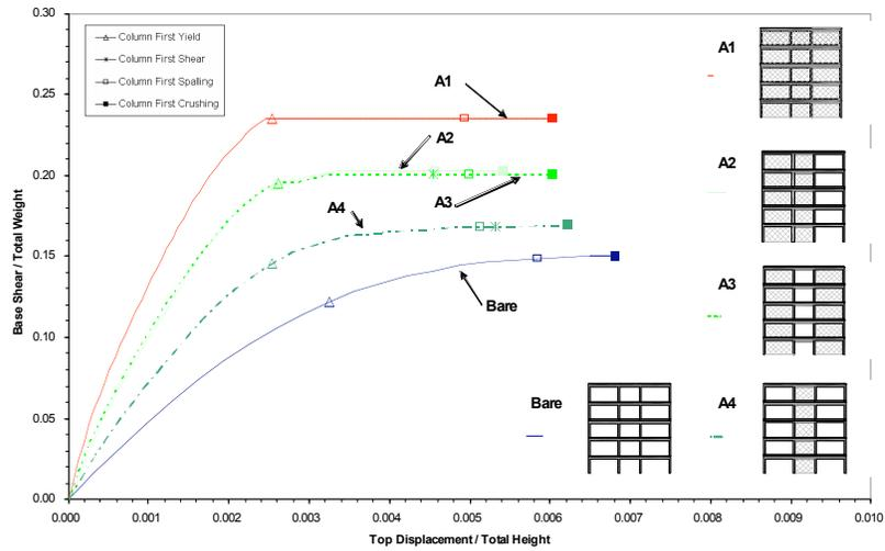
Fig. (21). Capacity curves – A series weak frame.
