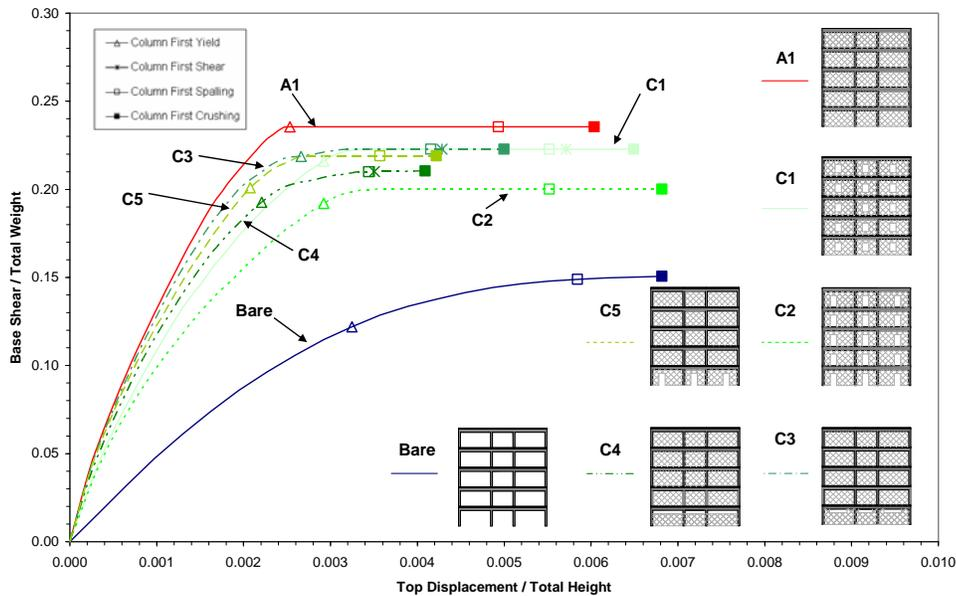
Fig. (27). Capacity curves – C series weak frame.
