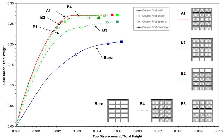
Fig. (23). Capacity curves – B series strong frame.
