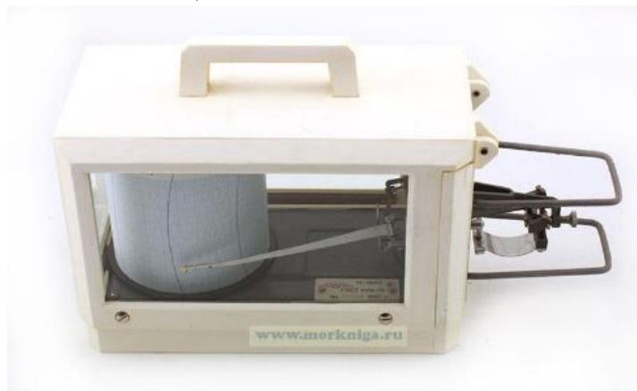
(e) weekly thermograph model M-16AN Thermograph.
