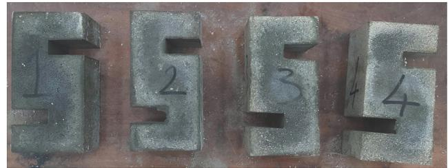
Fig. (5). Specimens prepared for shear strength testing.
