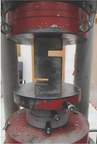
**Fig. (6).** Shear strength testing apparatus and setup.
