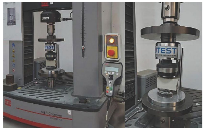
Fig. (2). Compressive strength testing apparatus.
