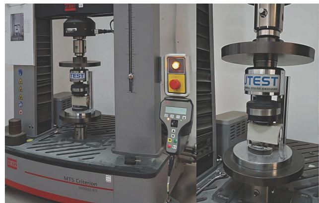
**Fig. (2).** Compressive strength testing apparatus.
