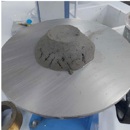
Fig. (1). Flow table test setup. Note: The photograph is intended to illustrate the test apparatus only and does not represent the actual flow result.
