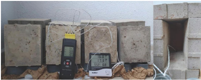
Fig. (7). Thermal performance monitoring setup.
