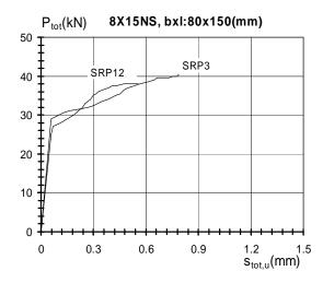
Fig. (9). Diagram of total force vs. total bond slip for  $8 \times 15$  specimens.
