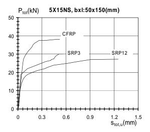
Fig. (8). Diagram of total force vs. total bond slip for  $5 \times 15$  specimens.
