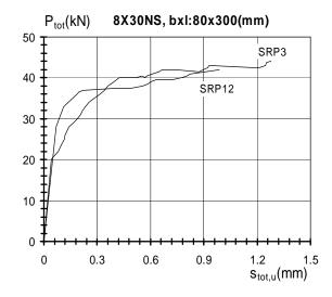
Fig. (11). Diagram of total force vs. total bond slip for  $8 \times 30$  specimens.
