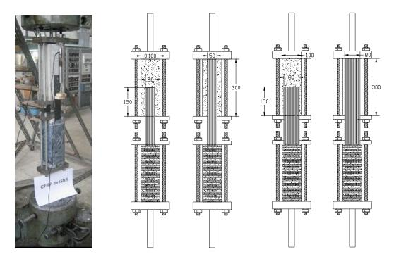
Fig. (6). Specimen ready for testing, and configurations of representative specimens.
