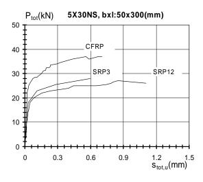
Fig. (10). Diagram of total force vs. total bond slip for  $5 \times 30$  specimens.
