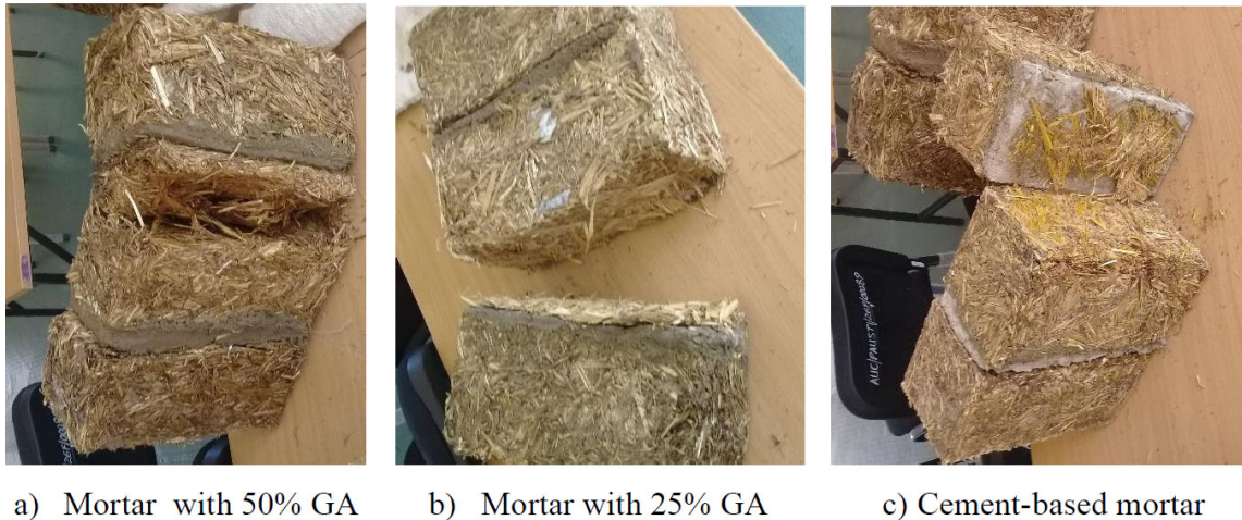
Fig. (5). Failure pattern of the prism.
