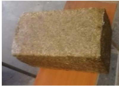
a) Block type 1 made of smaller size of chopped straw mixed with binder
