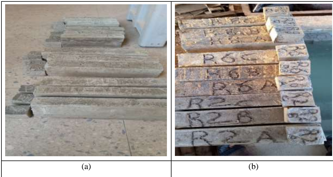
Fig. (6a,b). Samples of 100 mm concrete cubes and bamboo reinforced beams of 100×150×500 mm.
