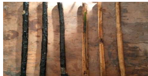
Fig. (3). Samples of coated and un-coated processed bamboo strips used as reinforcement.
