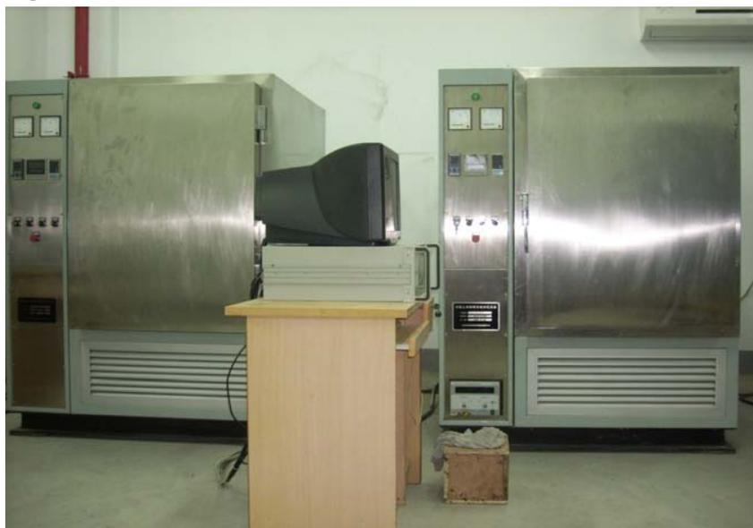
**Fig. (1).** Adiabatic temperature testing device.
